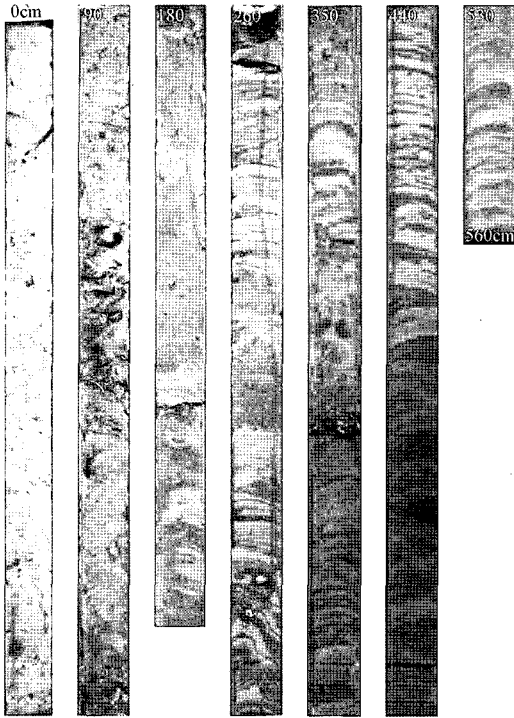
Fig. 9. Photographs showing core sediment sections of station #20. Sediments in the upper part of the core sample (0-150cm) are mixed with coarse grains and fine sediments (i.e., poorly sorted), and boulders are intercalated in the layer. In lower part of this core sample, there are numerous sediment layers such as parallel and cross laminae that can be easily found in the modern tidal flat environment.
