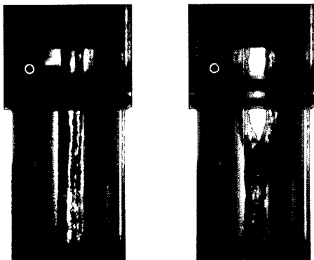
Fig. 9 Formation of air core in swirl chamber at L_s = 28 mm
