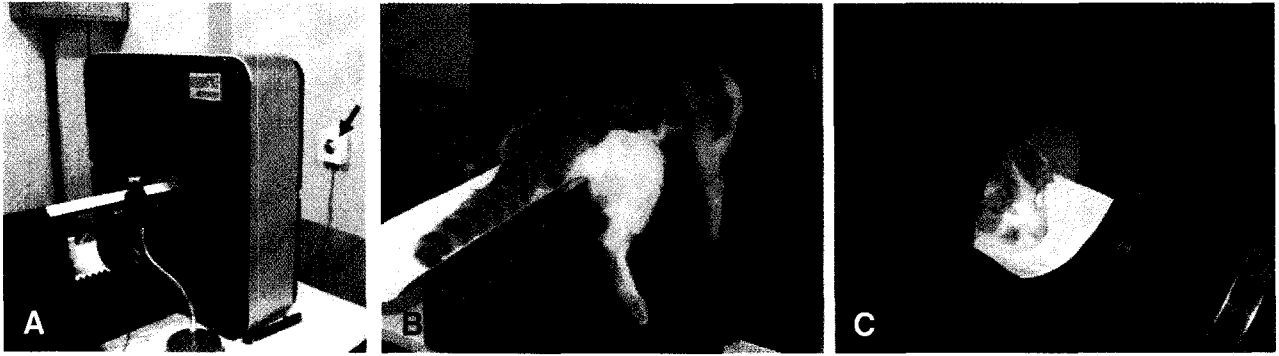
Fig. 1. (A) microPET R4 scanner (Concorde Microsystems Inc., Knoxville, TN). The position of cameras were indicated by the arrow. (B), (C) cat brain PET acquisition on the microPET R4 scanner.
