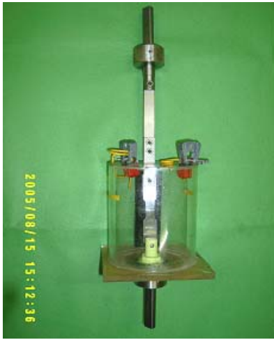
[Fig. 5] Chamber and connecting rod
