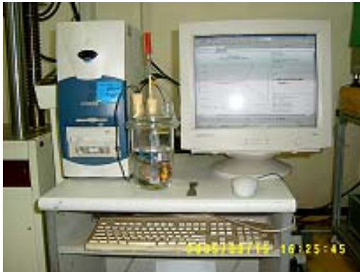
[Fig. 6] Schematic diagram of polarization test equipment
