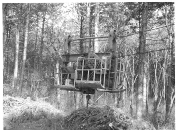
Figure 2. Self-propelled carriage used in stability analysis of cable yarding.
