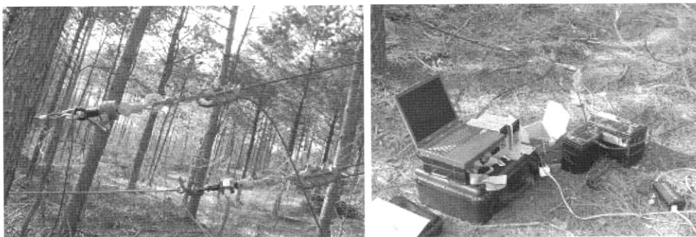
Figure 4. Load-cell and data acquisition system for measuring tension of wire rope.
