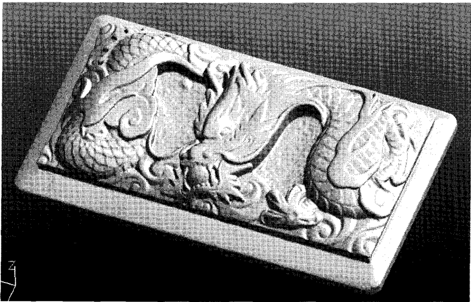
(b) view of polygon model after hole filling
