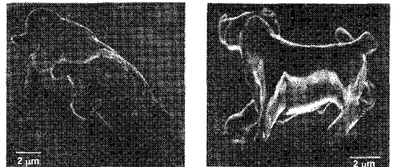
Fig. 16 Miniature statue of a bull fabricated by two-photon excited photopolymerization using femtosecond laser (Osaka University, Japan)
