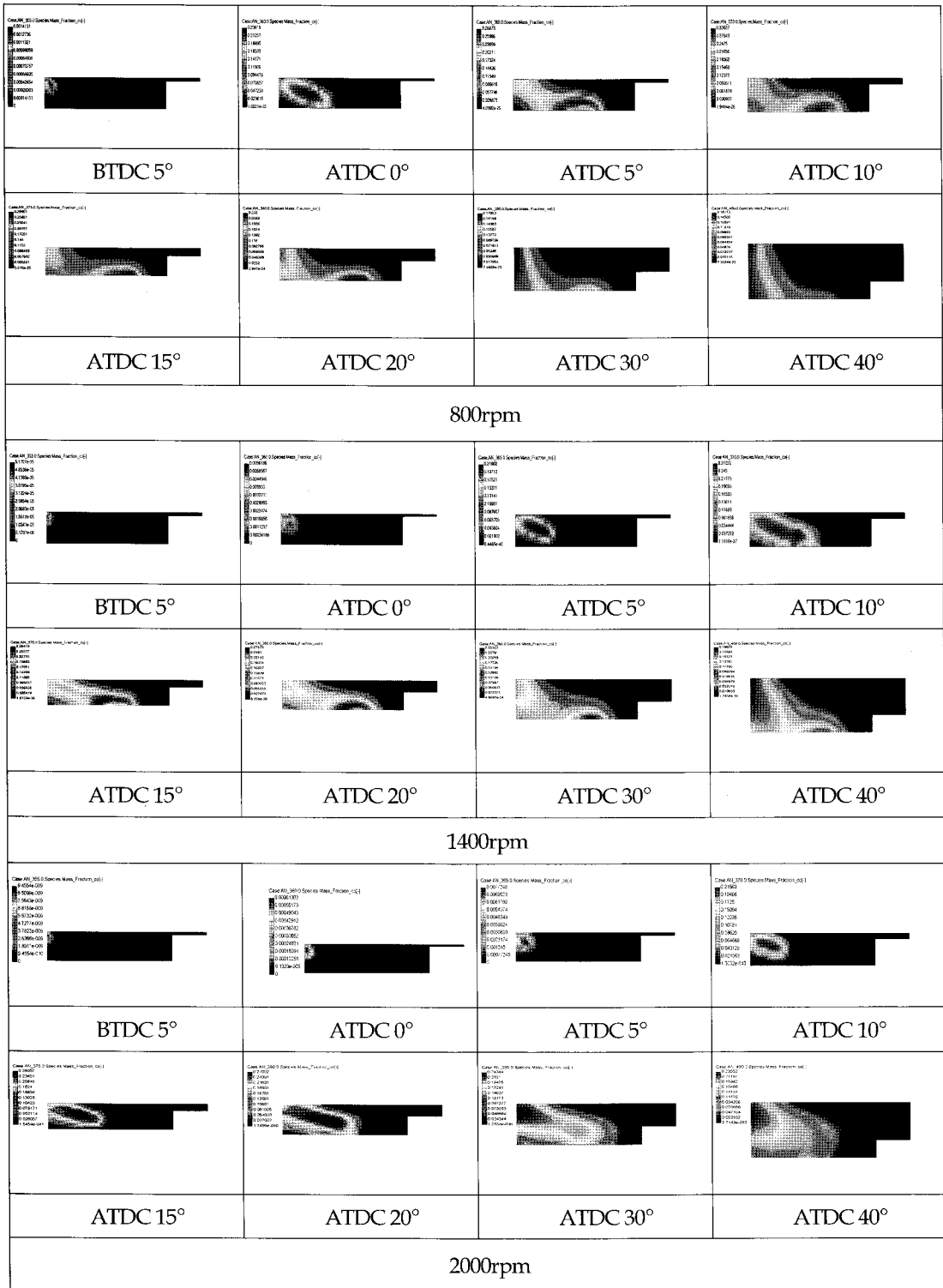
Fig. 8 Comparison of CO contours by engine speed
