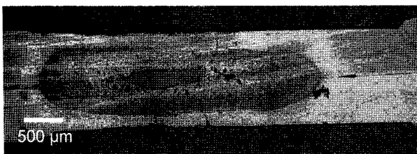
(b) Post-weld cold worked Al RSW (7.1 mm IS, 450 MPa IP)
