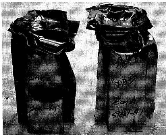
Figure 4. Deformed shape after the crush test.
