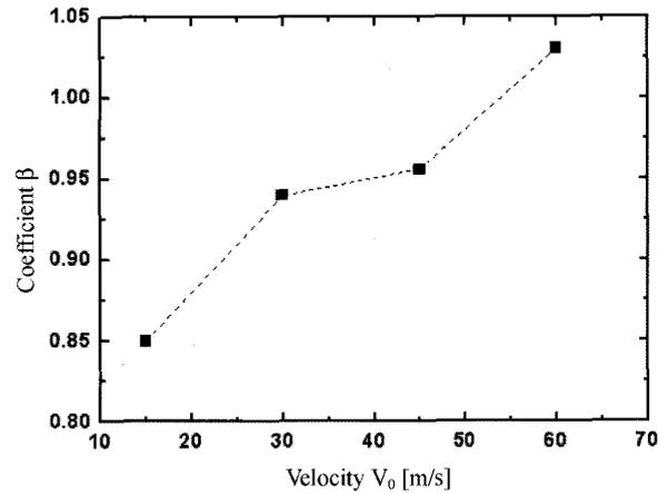
Figure 17. Estimated  $\beta\text{-}V_0$  curve for the viscoplastic model.
