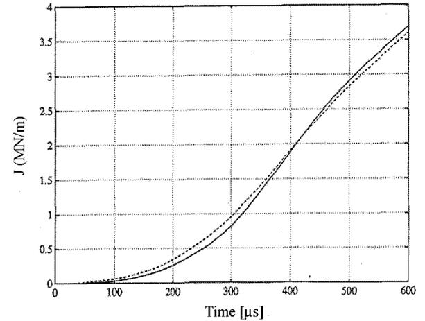
Figure 12. J-integral (solid line) and  $\beta(V_o)\sigma_y\delta_M$  (dashed line) history at the impact velocity of 60 m/s. ( $\beta$  is chosen as 0.76) in case of elastic-plastic material.
