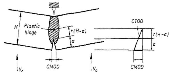
Figure 8. Plastic hinge, CTOD and CMOD.
