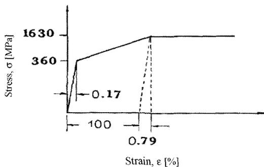
Figure 7. Static stress-strain curve of the material.
