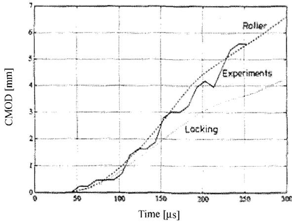
Figure 6. CMOD versus time at the impact velocity of 45 m/s for the two different simulations and the experiment (experiment: solid line, simulations, roller boundary: broken line, locking boundary: dotted line).
