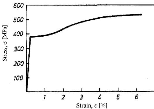
Figure 3. Static tensile test diagram.
