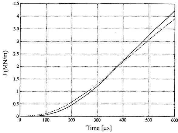
Figure 15. J-integral (solid line) and  $\beta(V_0)\sigma_y\delta_M$  (dashed line) history at the impact velocity of 45 m/s. ( $\beta$  is chosen as 0.98) in case of elastic-viscoplastic material.
