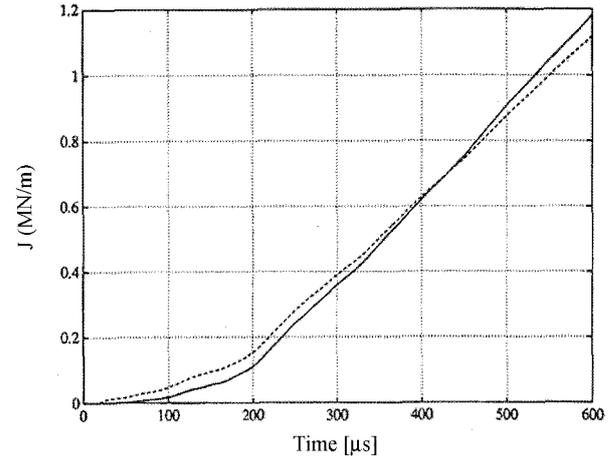
Figure 13. J-integral (solid line) and  $\beta(V_0) \sigma_Y \delta_M$  (dashed line) history at the impact velocity of 15 m/s. ( $\beta$  is chosen as 0.85) in case of elastic-viscoplastic material.
