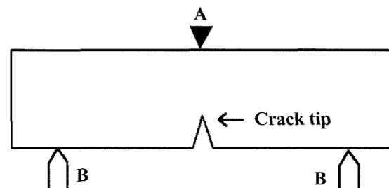
Figure 1. Geometry of the specimen.
