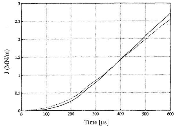
Figure 14. J-integral (solid line) and  $\beta(V_0) \sigma_Y \delta_M$  (dashed line) history at the impact velocity of 30 m/s. ( $\beta$  is chosen as 0.94) in case of elastic-viscoplastic material.
