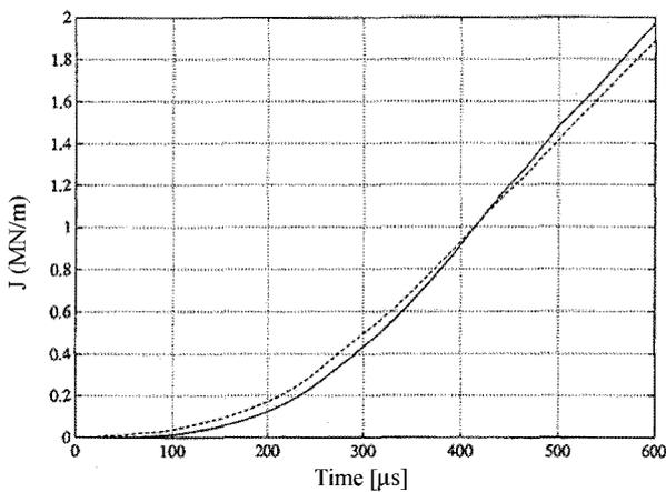
Figure 10. J-integral (solid line) and  $\beta(V_o)\sigma_y\delta_M$  (dashed line) history at the impact velocity of 30 m/s. ( $\beta$  is chosen as 0.76) in case of elastic-plastic material.
