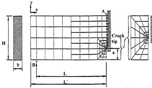
Figure 2. Finite element model for 3PB specimen with a quarter notch ( $L=300$  mm,  $L'=320$  mm,  $H=75$  mm,  $b=18$  mm,  $a=H/4=18.75$  mm).
