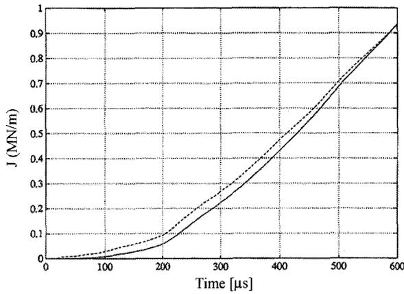
Figure 9. J-integral (solid line) and  $\beta(V_o)\sigma_y\delta_M$  (dashed line) history at the impact velocity of 15 m/s. ( $\beta$  is chosen as 0.76) in case of elastic-plastic material.
