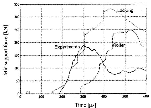
Figure 5. Mid-support force versus time at the impact velocity of 45 m/s for the two different simulations and the experiment (experiment: solid line, simulations, roller boundary: broken line, locking boundary: dotted line).
