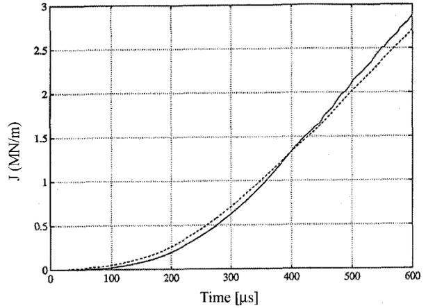
Figure 11. J-integral (solid line) and  $\beta(V_o)\sigma_y\delta_M$  (dashed line) history at the impact velocity of 45 m/s. ( $\beta$  is chosen as 0.76) in case of elastic-plastic material.
