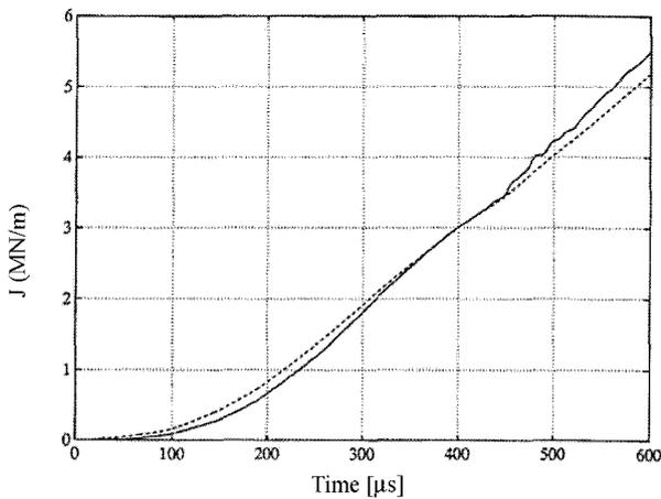
Figure 16. J-integral (solid line) and  $\beta(V_0)\sigma_y\delta_M$  (dashed line) history at the impact velocity of 60 m/s. ( $\beta$  is chosen as 1.03) in case of elastic-viscoplastic material.
