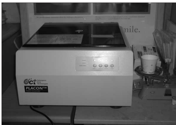
Fig. 3. The centrifuge for platelet concentration : PLACON®(Oscotec, Korea).
