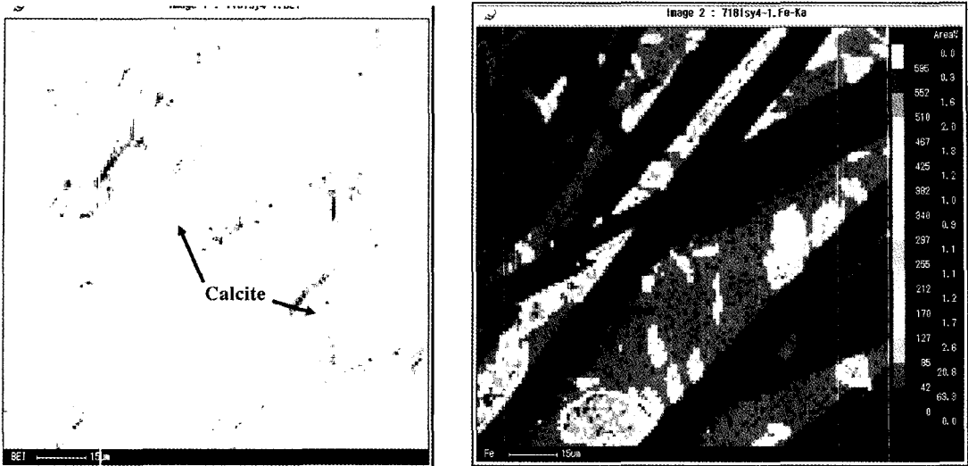
Fig. 4. EPMA mapping for the fracture secondary minerals such as calcite and iron oxides.
