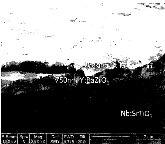
Fig. 6. SEM image of the BYZ film on the single crystal Nb:SrTiO 3 substrate (Sample#1 explained in the text). 35)
