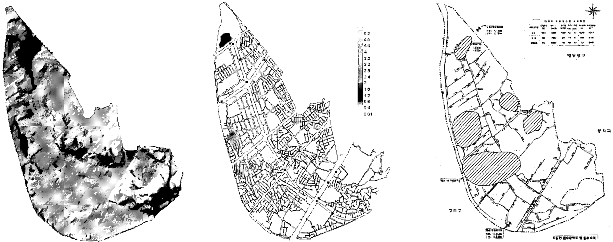
(a) Simulated Inundation Zones (level-pool Analysis) (b) Simulated Inundation Zones (2-D Maximum Flood Depth) (c) Surveyed Inundation Zones
