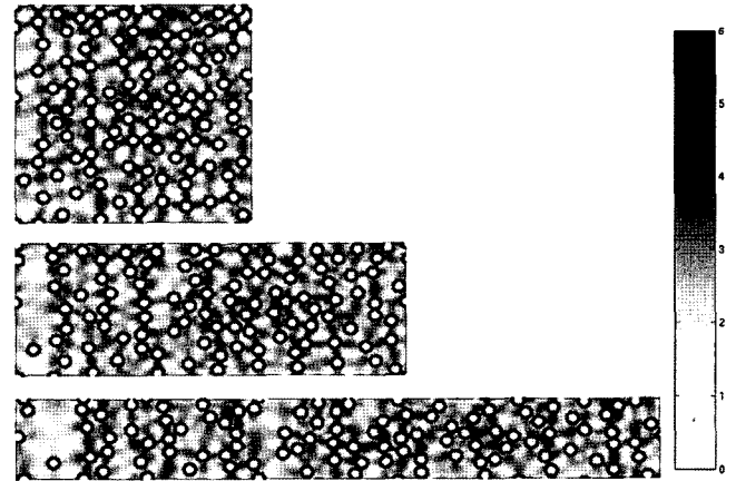
Fig. 8. An example 100 particle problem result for r=0.025 . The plotted quantity is the distribution of the shear rate \dot{\gamma}_{2D} : \dot{\varepsilon}t=0, 0.5 and 1 (from the top to the bottom). (Reproduced from Hwang and Hulsen, 2006).
