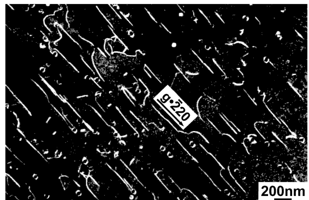
Fig. 12. Dark field micrograph showing dislocation loops in Ni24Al4Cr-0.5C alloy aged at 973 K for 1.08 Ms(300 h) and deformed 3% at 973 K.
