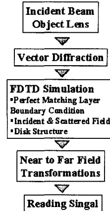
Fig. 2 Structure of FDTD simulator.
