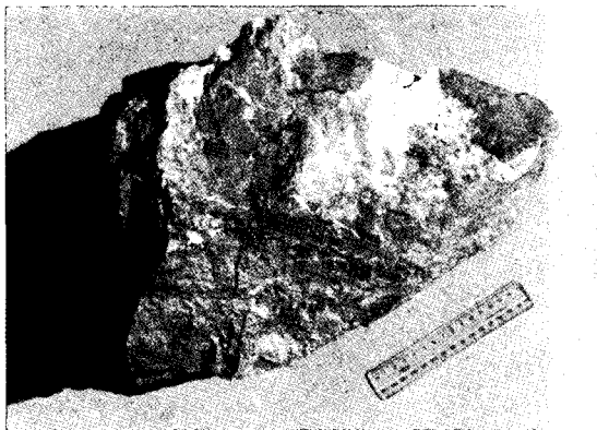
Fig. 6. Massive sulfide boulder, rich in chalcopyrite and sphalerite, recovered from strata-bound type mineralized volcanics.
