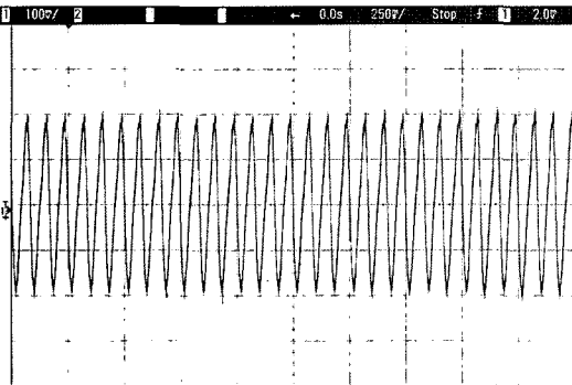
Fig. 7. The output voltage measured at 6Hz. The result was 198mV.
