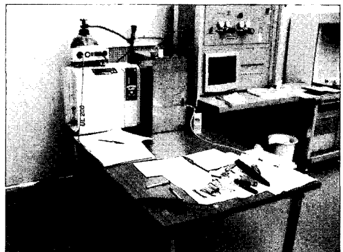
Fig. 12 Leakage Test Equipment
