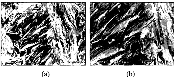
Fig. 8. SEM Images of 810°C heated tube at (a) x1000 and (b) x2000 magnification.
