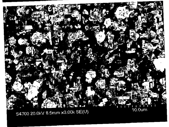
Fig. 5. SEM surface view of YBCO films deposited on a moving LAO (100) single crystal substrates with a speed of (a) 0.37 cm/min (b) 0.44 cm/min). Substrate temperature was 740 °C.
