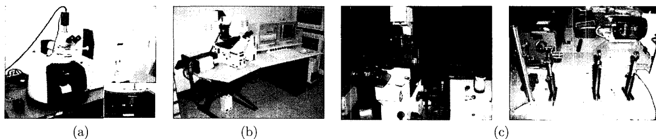
FIG. 4. Optical detection systems for microfluidic sensors: (a) confocal Raman microscope, (b) confocal laser scanning fluorescence microscope, and (c) confocal Raman/fluorescence microscope.
