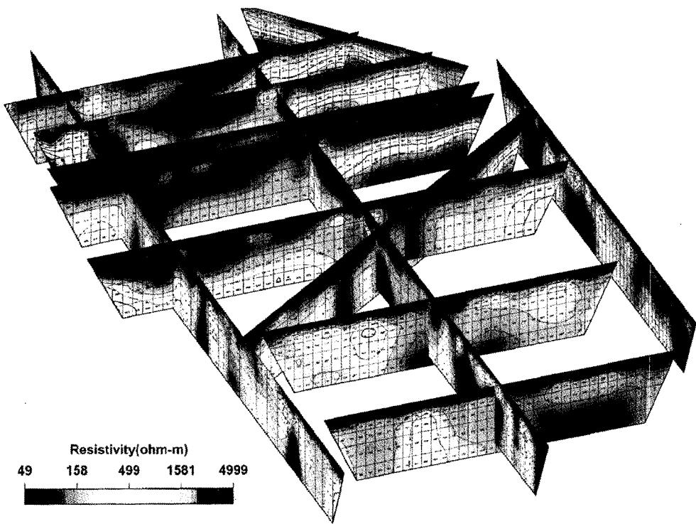
Fig. 7. Resistivity distributions of the fence diagram based on 2-D electrical resistivity survey.
