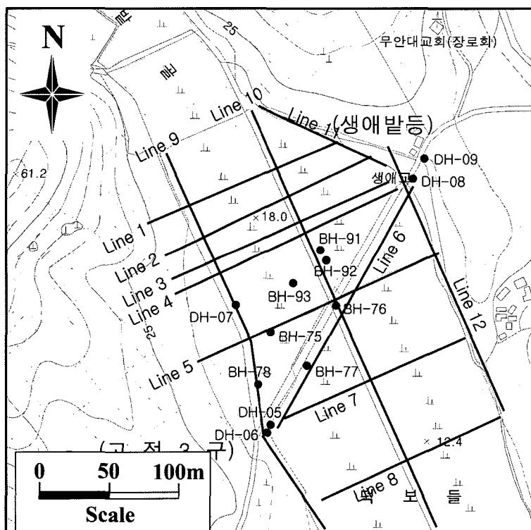
Fig. 4. Positions of boreholes and survey lines at the field site.
