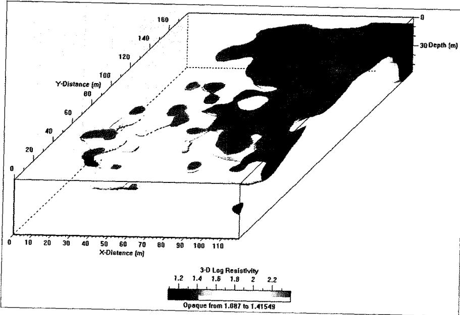
Fig. 11. Underground cavities imaging from 3-D electrical resistivity survey.
