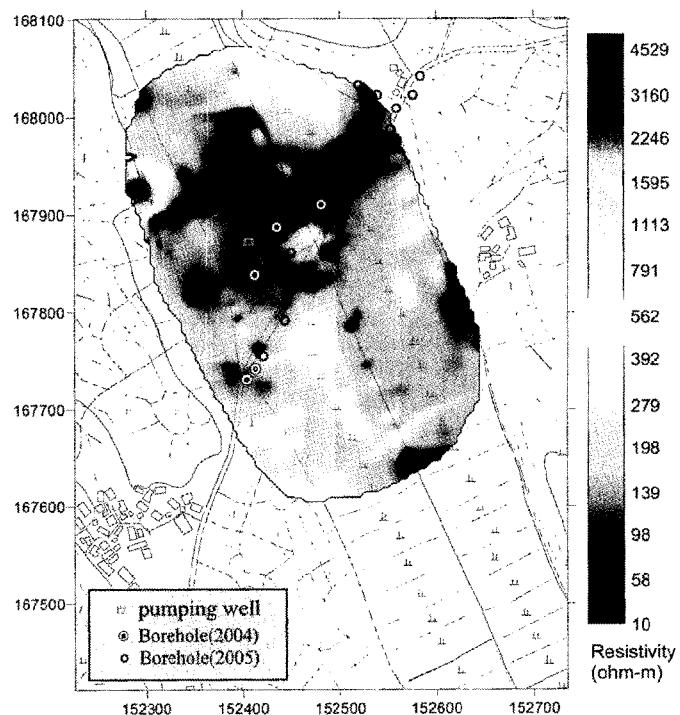
Fig. 8. Slice of resistivity distribution at 10 m depth.
