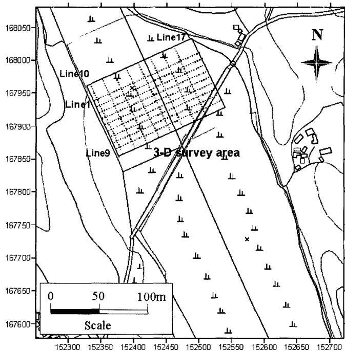
**Fig. 9.** 3-D electrical resistivity survey area in the field site.
