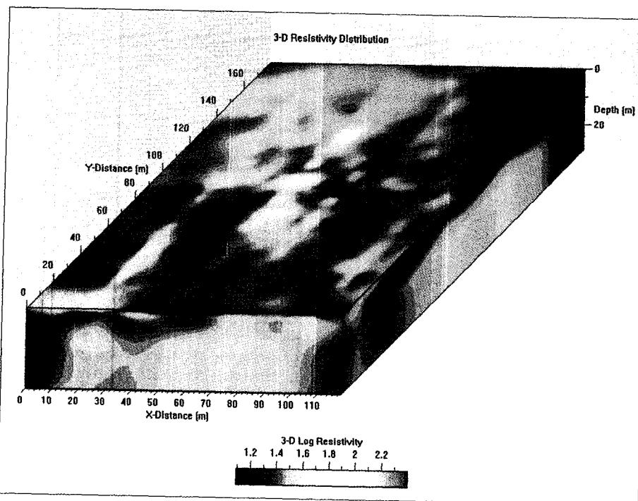
Fig. 10. 3-D resistivity distribution of the survey area.
