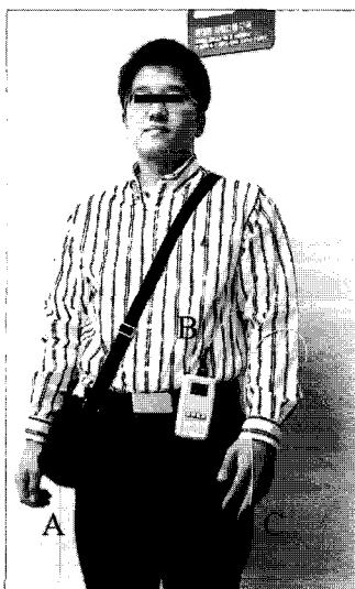
Fig. 10. Total ubiquitous SaO 2 monitoring system. A: Small bag containing transmission unit, B: Measurement unit, C: Finger clip sensor
