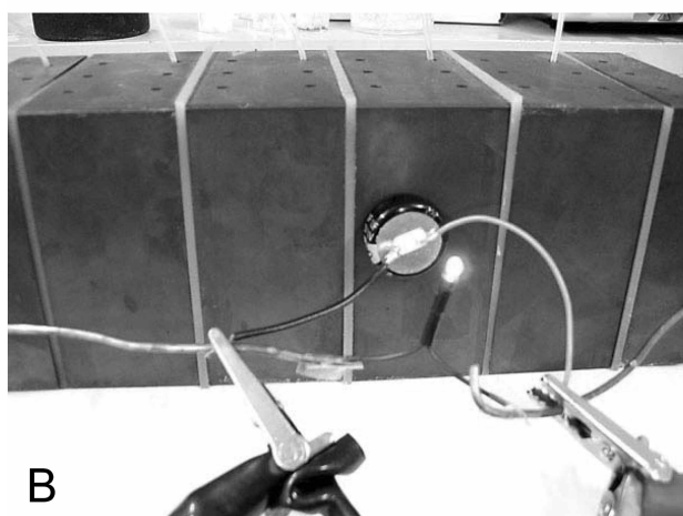
Figure 5. MFC output voltage change as a function of time (panel A) and the picture of powering of an electric bulb (panel B) from electricity stored in a 1 F supercapacitor.
