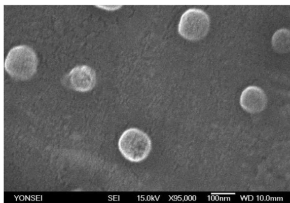
Figure 15. SEM image of the capsules formed by 20 ( 5 \times 10^{-3} g/mL) in \text{H}_2\text{O} in the presence of \text{CHCl}_3 ( 1 \times 10^{-2} mL/mL).
