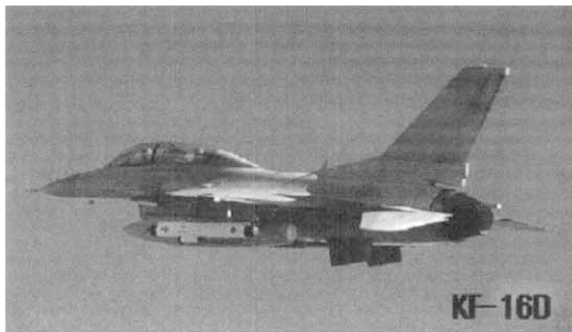
Fig. 11. Flight Test of KF-16D with ALQ-X Pod
