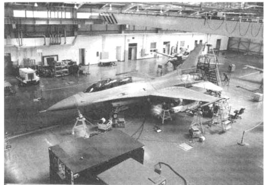
Fig. 9. Ground Vibration Test of KF-16D
