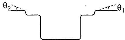
Fig. 10 Definition of the flange shape change after the springback
