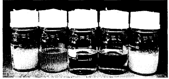
Fig. 8 Solubility of PC pellet in THF and DMF (THF:DMF=100:0, 90:10, 80:20, 40:60, 0:100 left to right at 25 °C)
