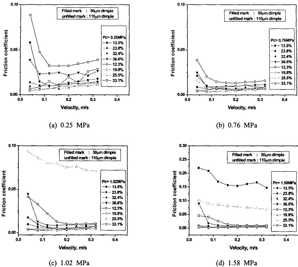
Fig. 6 Friction coefficient as a function of velocity on 50 $\mu\text{m}$  and 110 $\mu\text{m}$  of micro dimples
