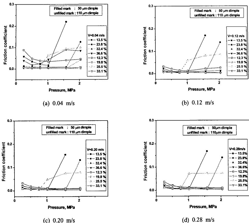
Fig. 5 Friction coefficient as a function of pressure on  $50 \mu\text{m}$  and  $110 \mu\text{m}$  of micro dimple
