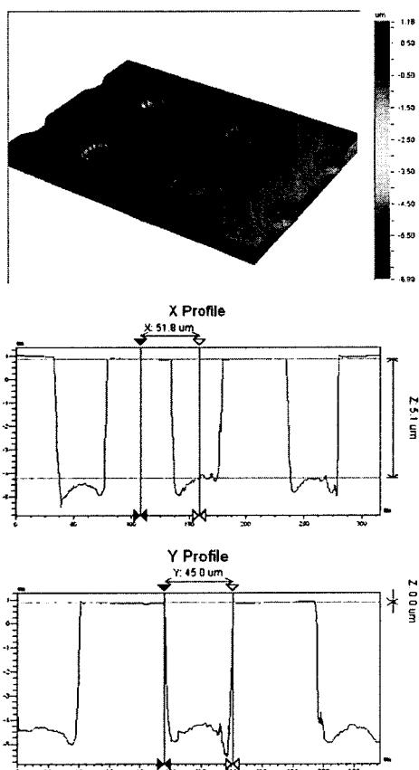
Fig. 1 The surface topography and profile for 50  $\mu\text{m}$  dimple
