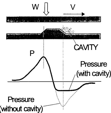
Fig. 9 Hydrodynamic mechanism for surface texture.
