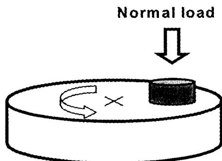
Fig. 4 Schematic illustration for pin on disk
