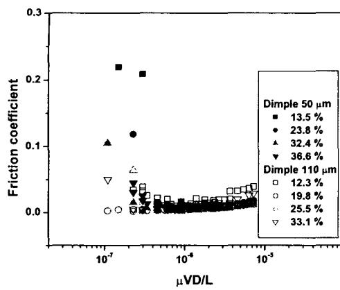
Fig. 7 Stribeck curves on  $50 \mu\text{m}$  and  $110 \mu\text{m}$  of micro dimples
