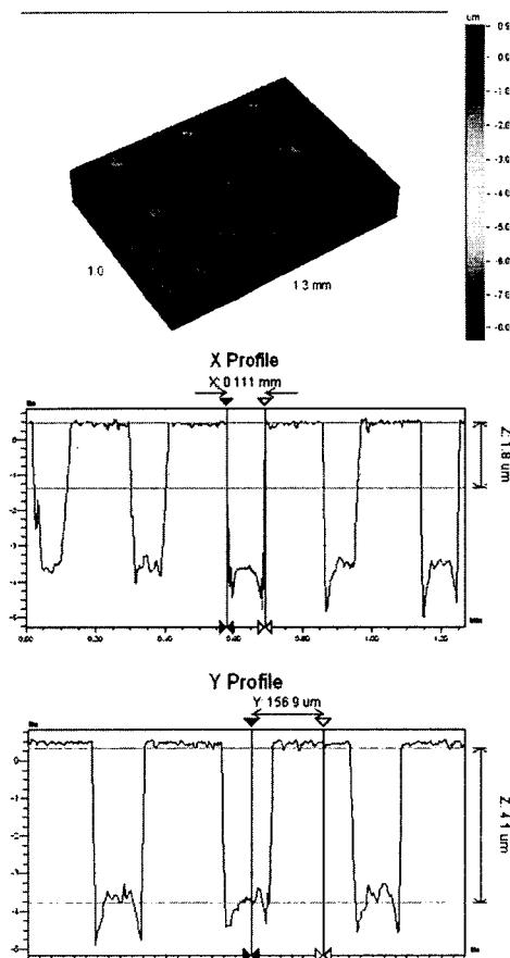
Fig. 2 The surface topography and profile for 110  $\mu\text{m}$  dimple
