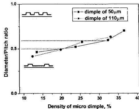
Fig. 10 Diameter/Pitch ratio as function of density of dimple for 50  $\mu\text{m}$  and 110  $\mu\text{m}$
