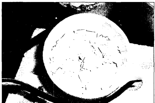
Fig. 3. The melting sample of aluminum with flux B or C.
