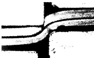
Fig.14 Shearing process of anti-vibration sheet metal in case of clearance 20%
