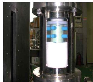
그림 9 Picture of filling the bottle with 70 Percent of beads.
