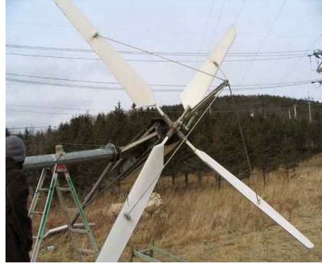
Fig. 2 Blade damper with 4 bars.
