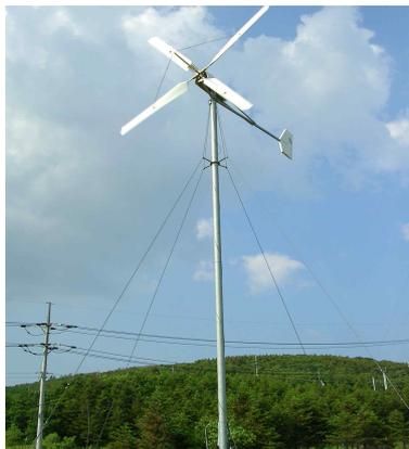
Fig. 1 6kW W/T test model.
