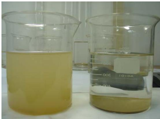
Fig.9 Treatment Result for Turbid Water of DOAM Dam
