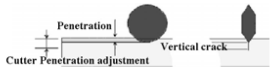
Fig. 2 Principle of vertical crack
