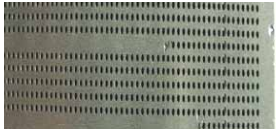
Fig. 3 Workpiece after hole drilling
