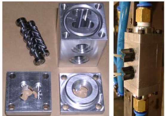
Fig. 9 Development of screw flowmeter
