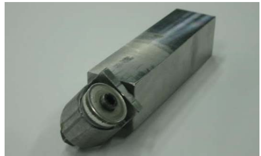
Fig. 2 Rotary tool holder
