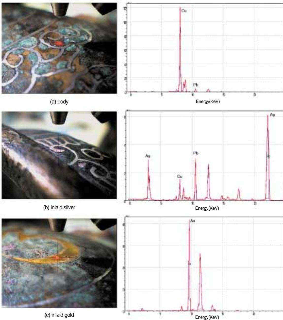
Photo 3. The process of analysis and XRF spectrum of the surfaces
