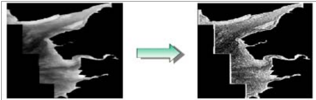
FIGURE 9. KOMPSAT EOC image conversion using high frequency pass filtering for tidal flat extraction(Seo han bay, North Korea, 2001.9.18)
