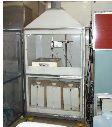
Fig. 1. Photographs of the laboratory pickling test equipment.
