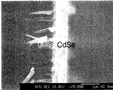
Fig. 1. SEM images of CdSe films at magnification of 20,000 and the cross sectional view of glass/CdSe.
