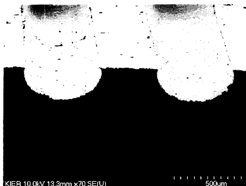
(a) Micro channel patterned plate
