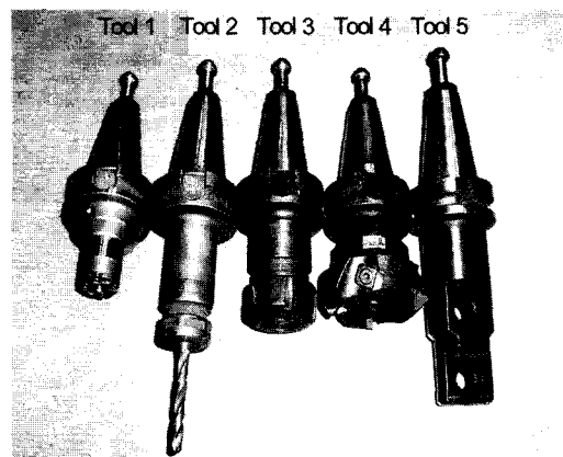
Fig. 11 Tool and tool-holder models for experiment
