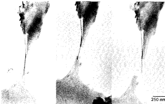
Fig. 17. A weak interaction between the epoxy matrix and the nanotube leads to pull-out.
