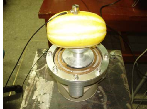
Fig. 3. Arrangement of vibration shaker, intact oriental melon and accelerometer.
