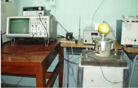
Fig. 2. General view of the sweep vibration apparatus for the oriental melon.
