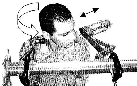
Fig 1. Apparatus and set-up for proprioceptive sensitivity testing. The arrows indicate the moving directions of the shaft driven by the stepper motor. The subject shown is making a left cheek contact with the moveable plate attached to the stepper motor after a left rotation movement. The right cheek was in contact with the fixed black rubber knob to define the start position for the movement. Visual focus was maintained as directly ahead during rotation movements.
